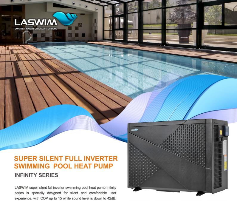
LASWIM super silent full inverter swimming pool heat pump Infinity series is specially designed for silent and comfortable user experience, with COP up to 15 while sound level is down to 42dB. Thanks to the DC inverter compressor, stepless inverter control system and brushless fan motor, the speed can be adjusted Hz by Hz and round by round, to achieve energy saving and super silence.
